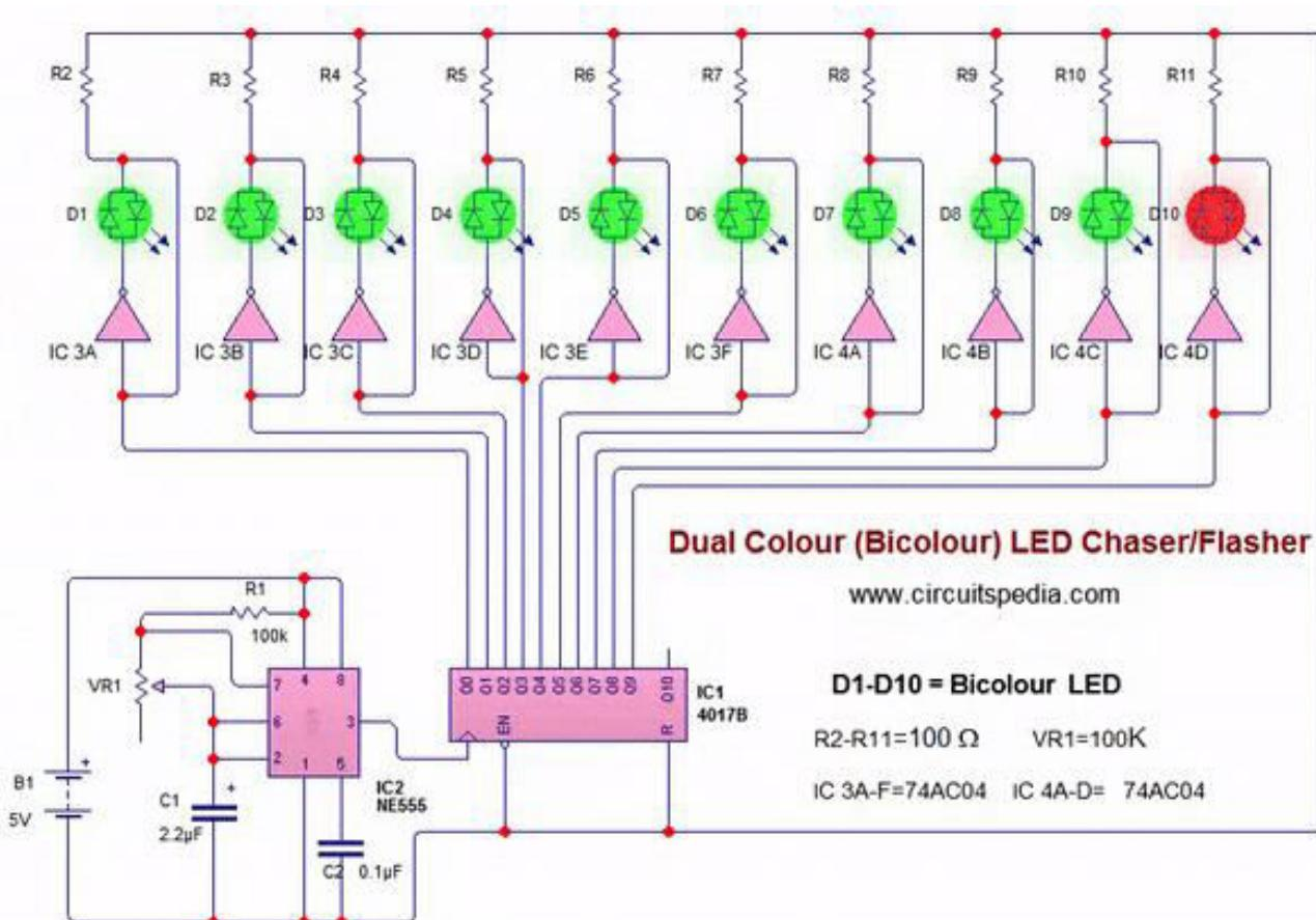
Here I am presenting a circuit of 10 dual colour LED flasher (Not using Flashing LED) which blinks one by one in sequence. This circuit is based on popular counter circuit using [4017](#) and [555](#).
